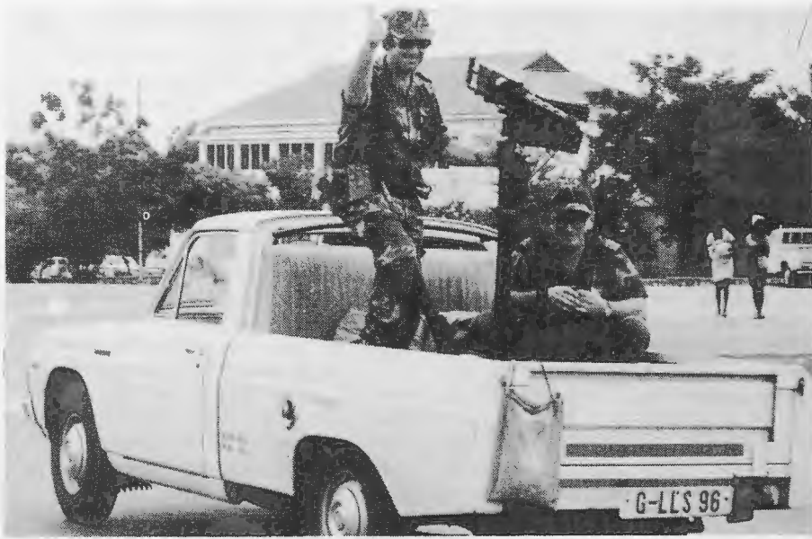
Datsun pickup used as "gun jeep" to accompany convoys carries MAG light machine gun manned by members of BSAP Reserve.
